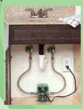
is needed, the pump is activated by pressing a starter button, runs only long enough to supply hot water to the fixture and then automatically stops. This prevents hot water from entering the cold line. A spring-loaded Integral Flow-Check valve (IFC®) prevents cold water from entering the hot line. Optional wireless RF or motion sensor starters are also available.
