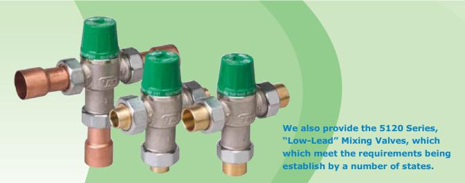
The 5000 Series Mixing Valve is a dual purpose mixing or diverting valve. It is ASSE 1017 approved, providing shut-off reliability on either a hot or cold water supply failure. The high flow and low headloss characteristics make the 5000 Series ideal for domestic water, radiant applications, installations with large variations in flow rate and supply conditions, and installations requiring tightly controlled water temperature.
