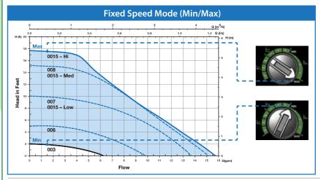
Fixed speed mode allows the installer to fine tune the circulator flow rate to precisely match design load conditions. It is infinitely variable between min/max settings.
