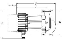
\* Controller Module standard on -FC1A01 models. Adds 1-5/16" to dimensions B and C.
