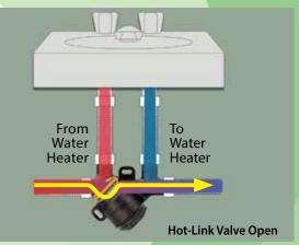
LEFT: No under-sink electricity needed. The Hot-Link Pump is mounted at the water heater.
