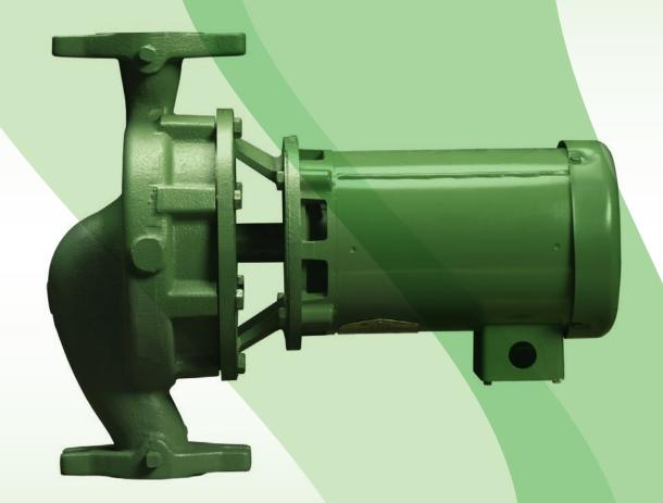
The Taco 1900 Series Close-Coupled In-Line Pumps are designed to be energy efficient and fit anywhere in the piping layout. The 1900 Series is self supported by the piping and can be installed horizontally or vertically. The pump and sealed ball bearing motor a re maintenance free. Rear pull-out design and standard motor simplify servicing and a single seal and shaft sleeve fits all models.
