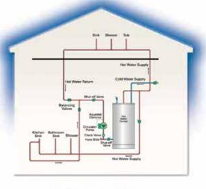
Recirculation Piping with Indirect Water Heater
