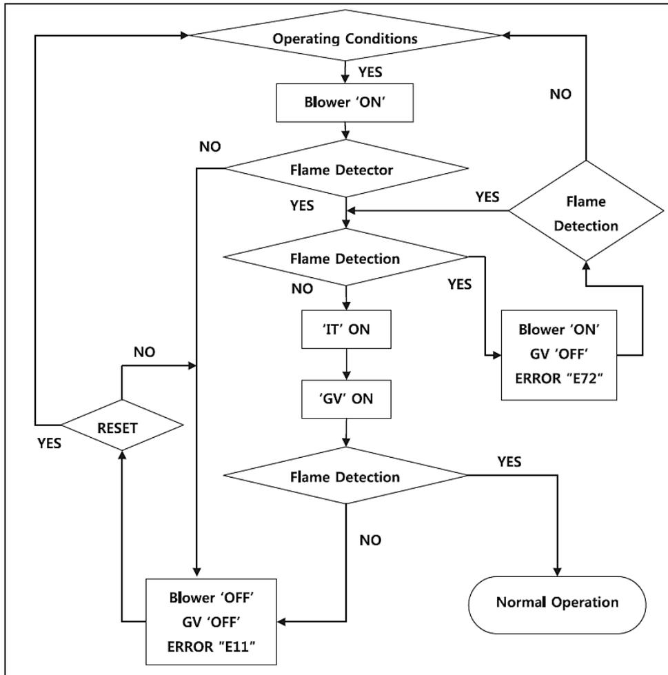
Figure 43 – Flame Detection Error Analysis Tree
