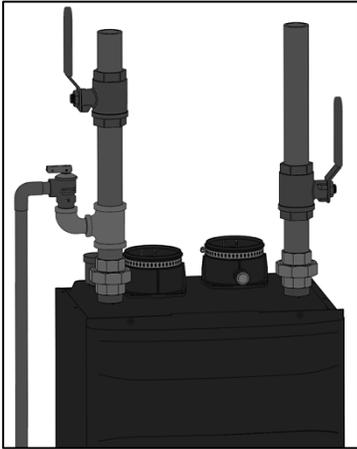
**Figure 26 – Pressure Relief Valve**
