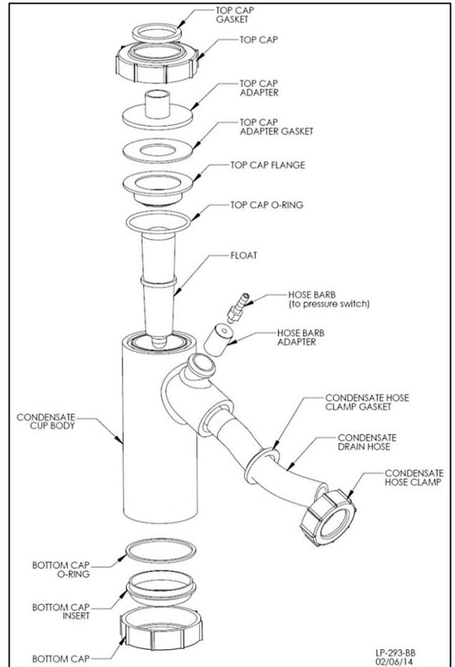
**Figure 52 – Condensate Detail**
