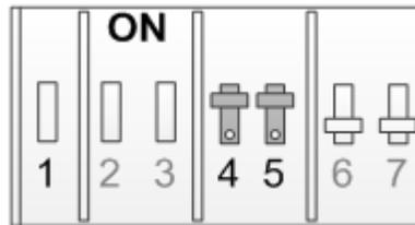
Figure 30 – Factory Default Dip Switch Detail
