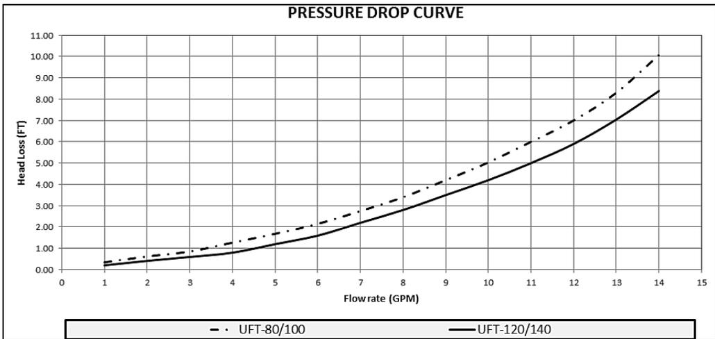
**Table 15 – Pressure Drop through the Heat Exchanger**
