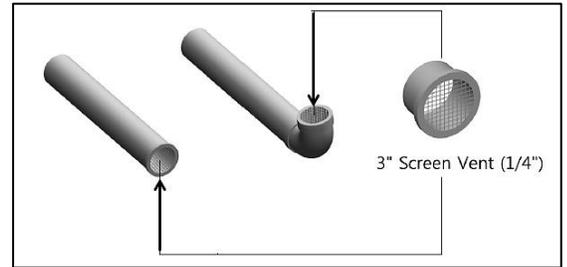
Figure 12 - Screen Installation
