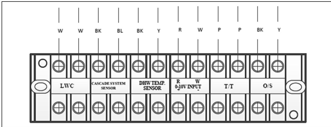
Figure 34 – Low Voltage Wiring Detail
