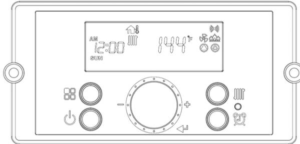
**Figure 37 – Initial Display Screen Example**
