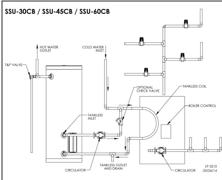
**Figure 3 - Typical Storage Tank Installation - SSU-30CB - SSU-60CB Models**
