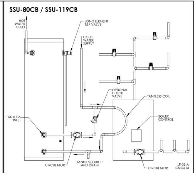
**Figure 4 - Typical Storage Tank Installation - SSU-80CB and SSU-119CB Models**
