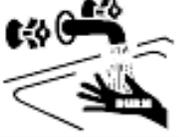
Water temperature over 125 degrees F. can cause severe burns instantly, or death from scalds. Children, disabled, and elderly are at highest risk of being scalded. See instruction manual before setting temperature at water heater. Feel water before bathing or showering! Temperature limiting valves are available. See chart below showing temperature burn rate.
