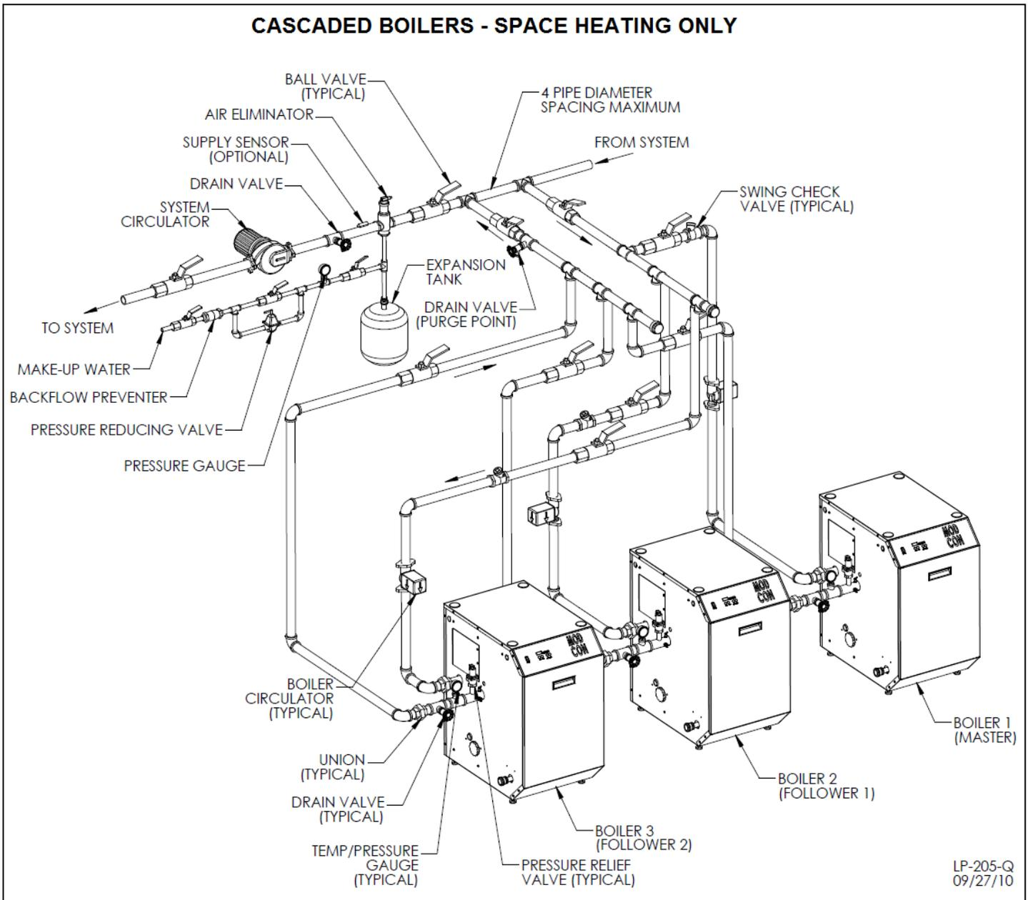
**Figure 11 – Cascaded Boilers – Space Heating**
