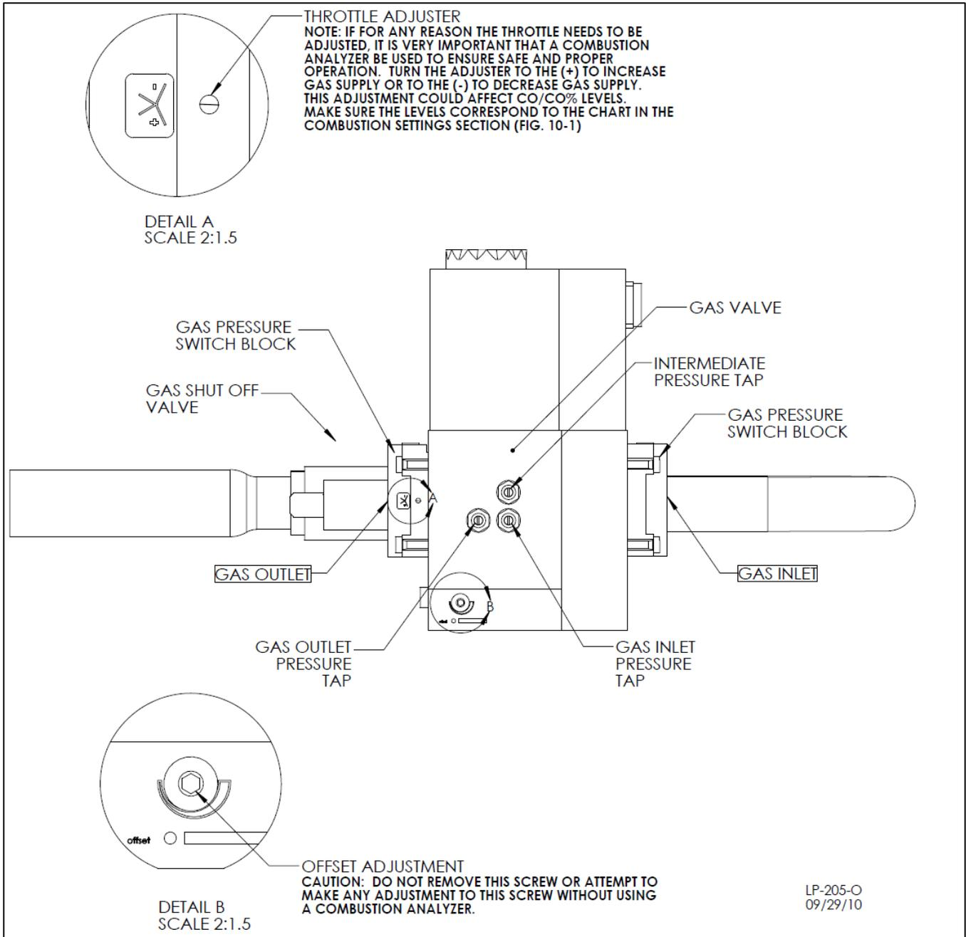
Figure 21 – Mod Con 850 Gas Valve
