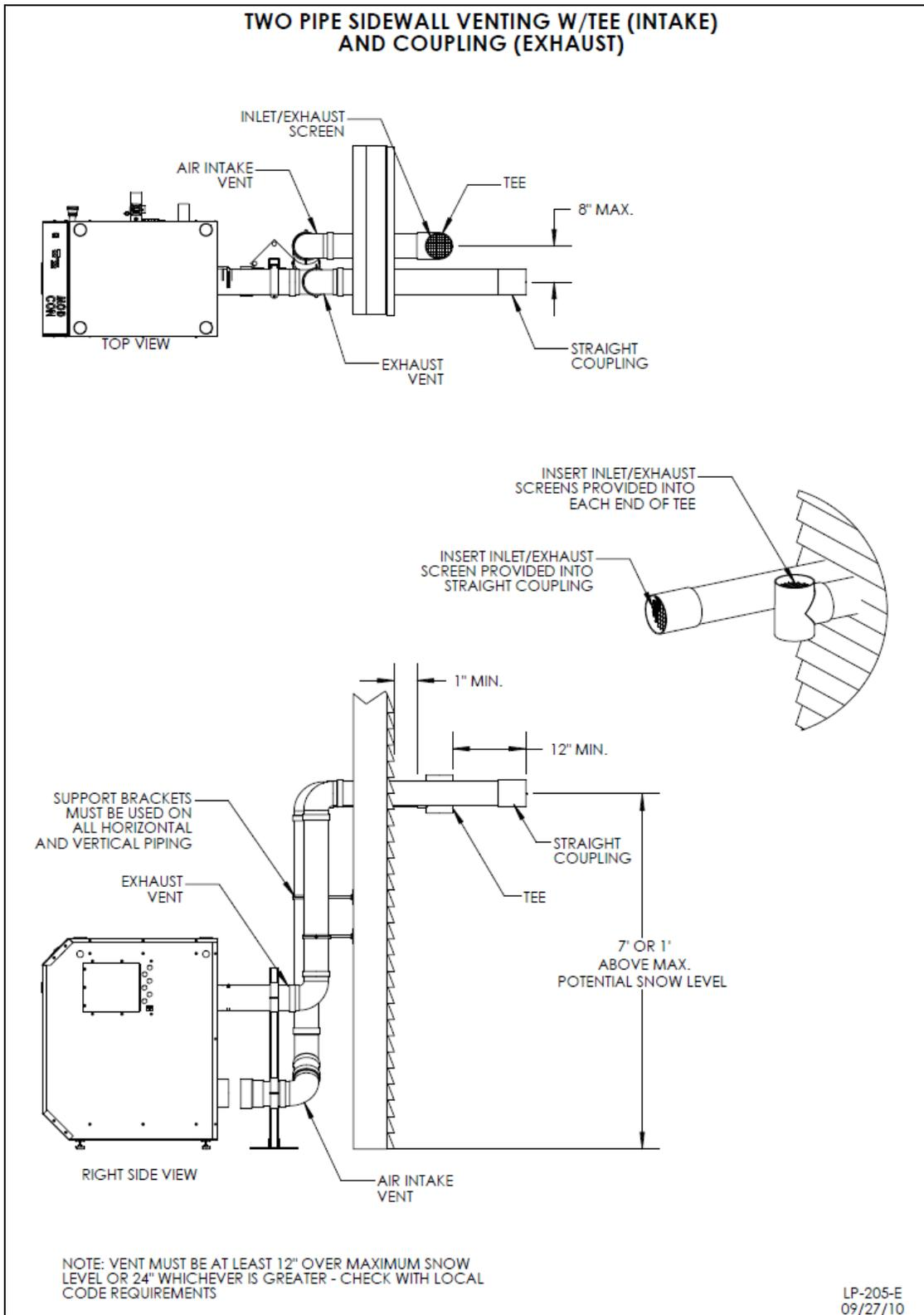
**Figure 16 – Sidewall Venting with Tee and Coupling**
