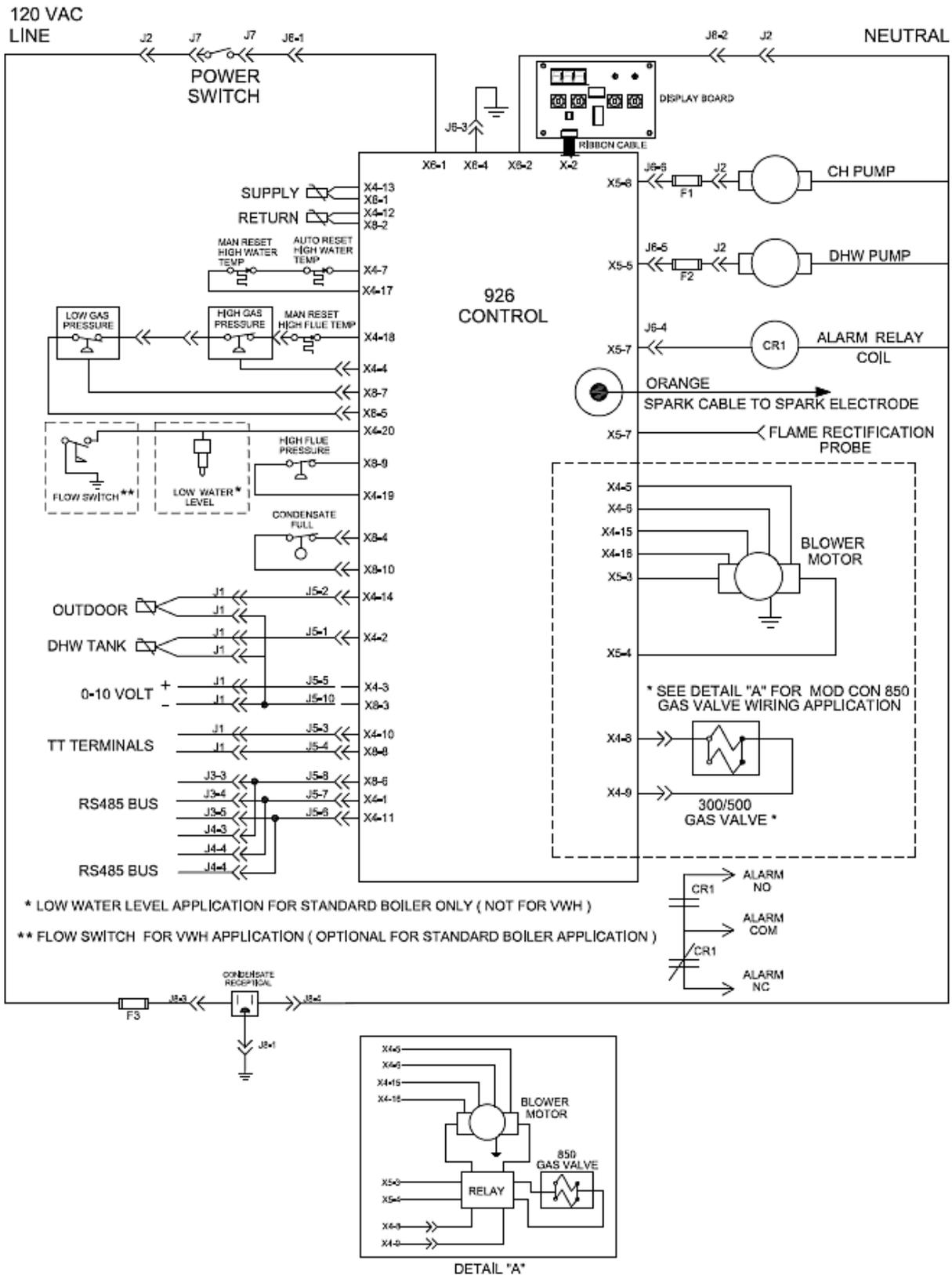
Figure 27 – Mod Con Internal Connection Diagram
