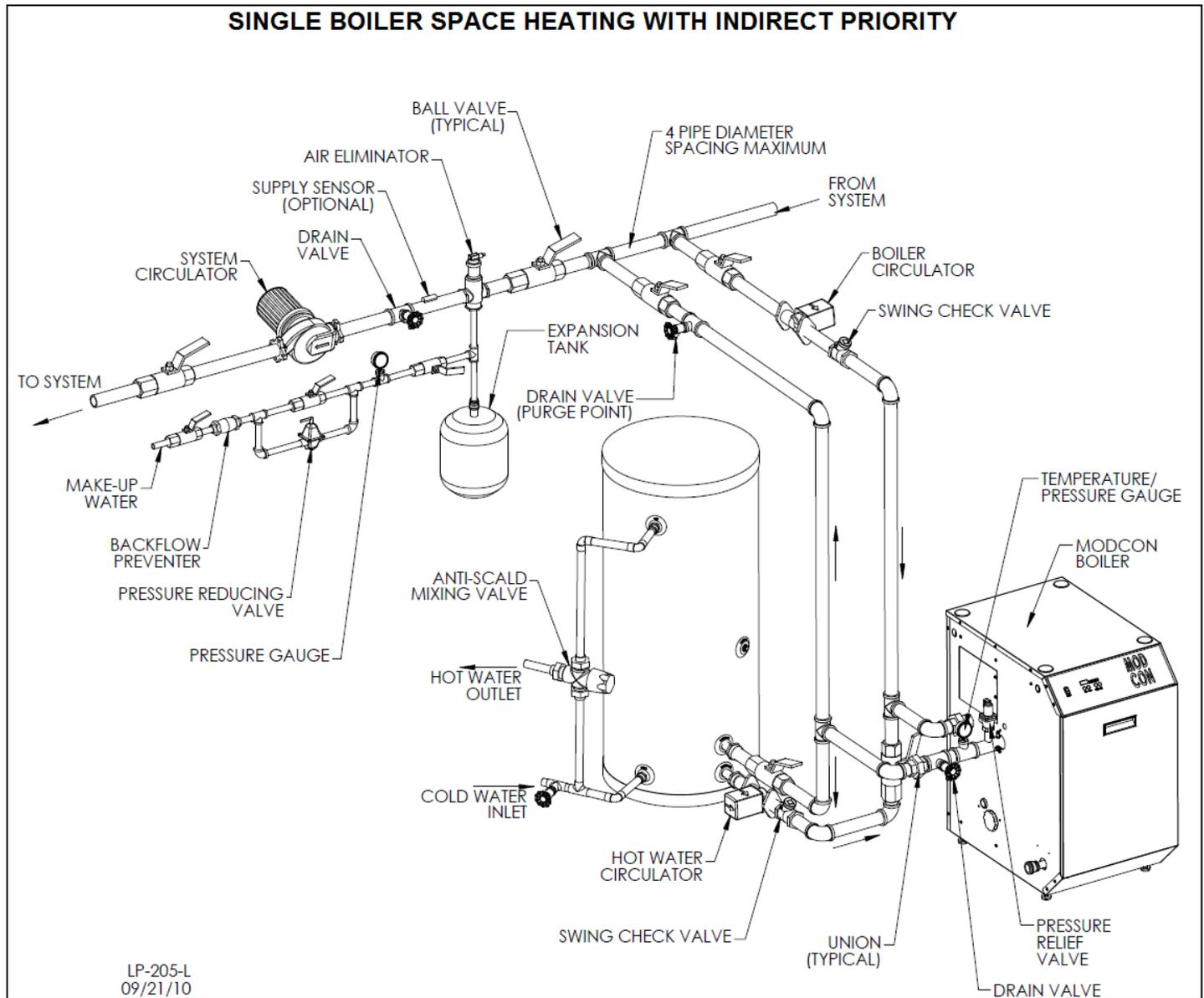
**Figure 8 – Single Boiler Space Heating – Indirect Priority**
