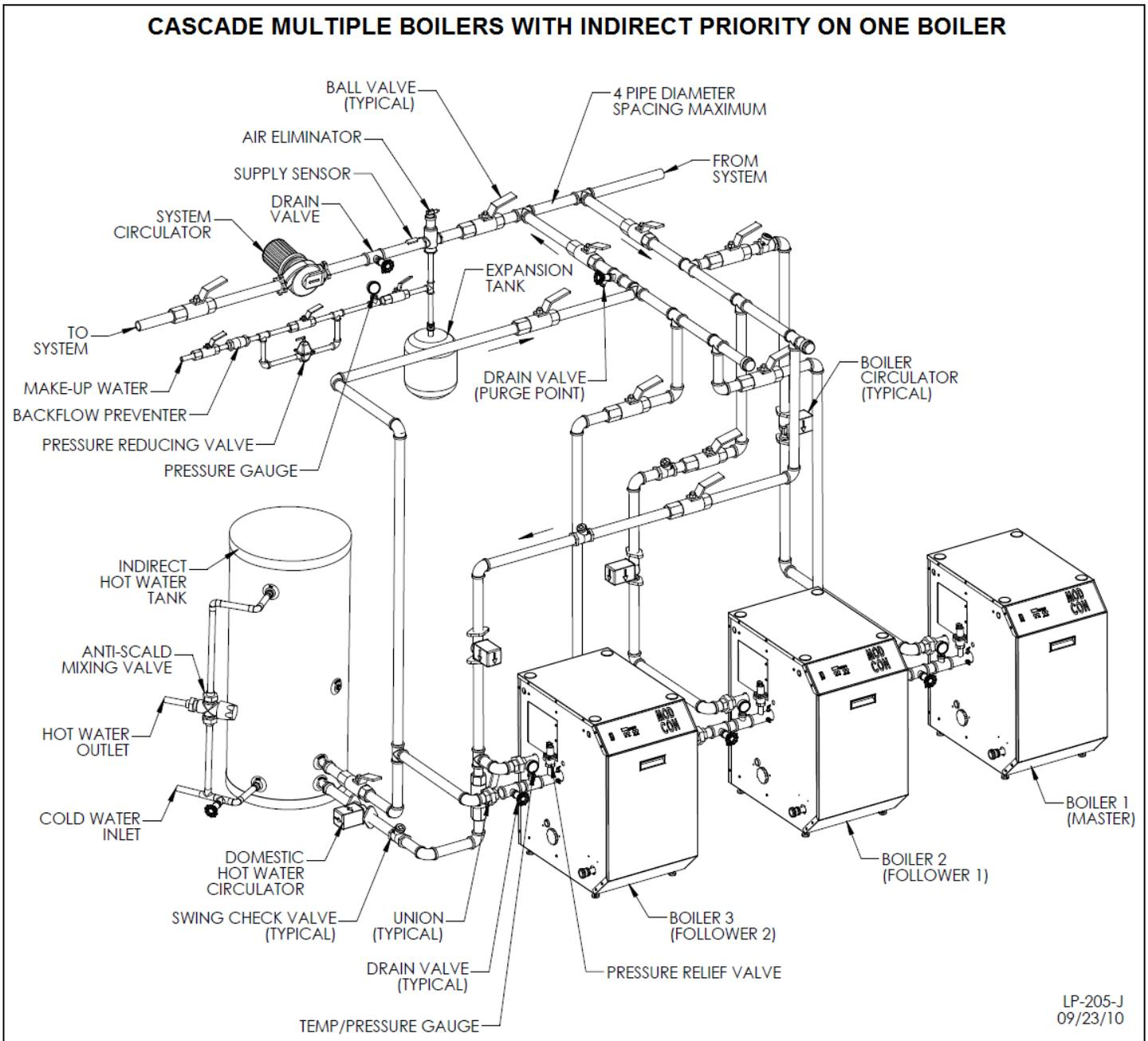
**Figure 9 – Cascade Multiple Boilers – Indirect Priority on One**
