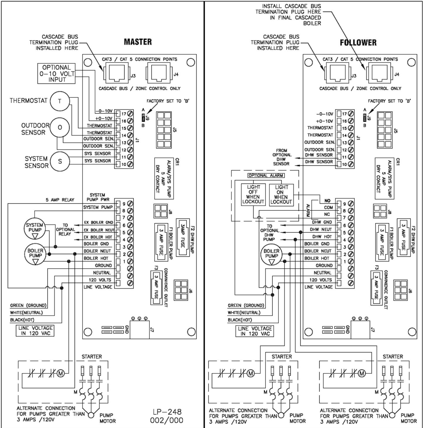
Figure 26 – Mod Con Cascade Master and Follower Wiring
