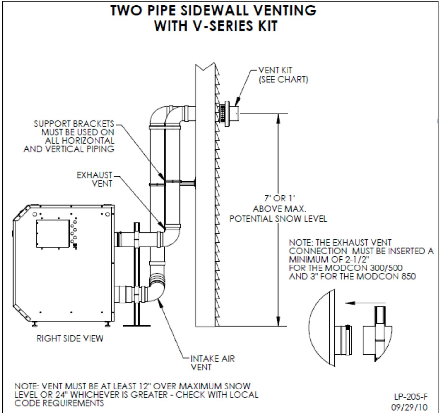
**Figure 15 – Sidewall Venting Diagrams**
