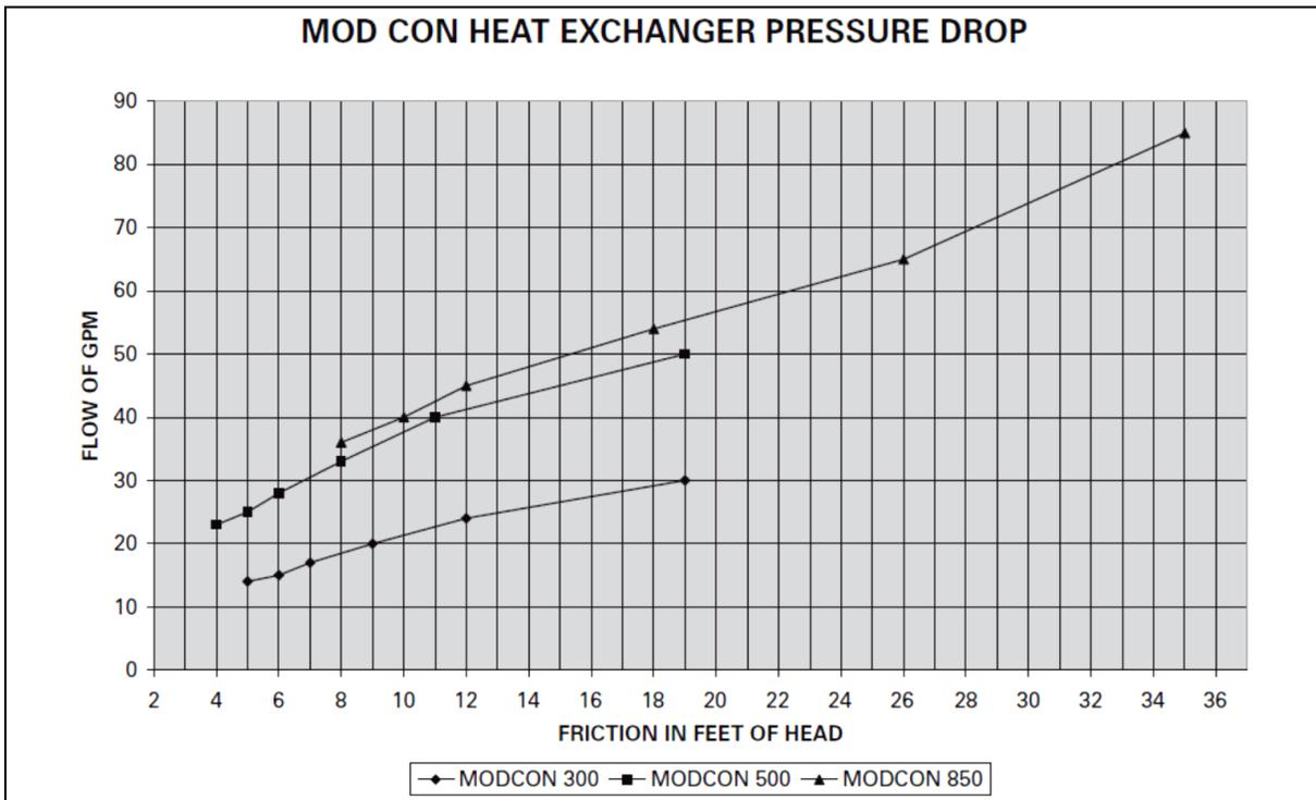
**Figure 6 – Heat Exchanger Pressure Drop Chart**
