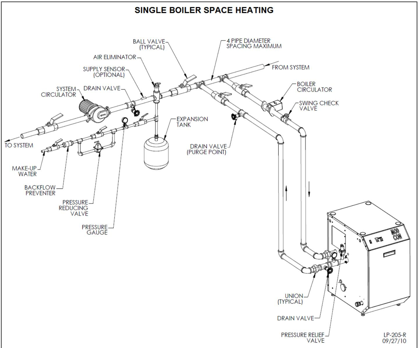
**Figure 10 – Single Boiler Space Heating**
