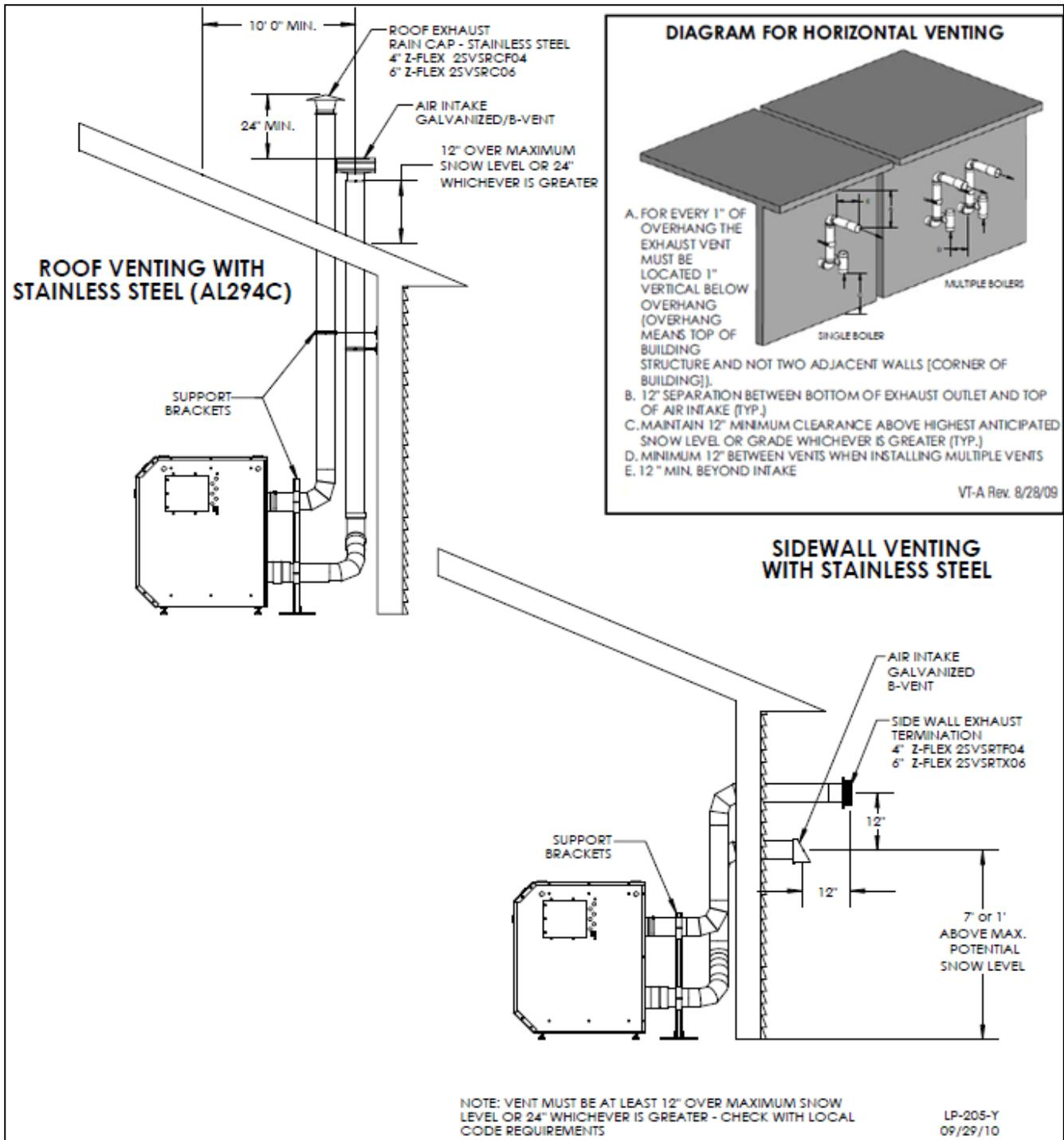
Figure 18 – Roof and Sidewall Venting with Stainless Steel
