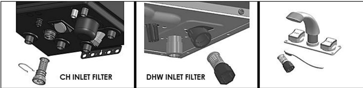
**Figure 50 – Cleaning the Inlet Filter**
